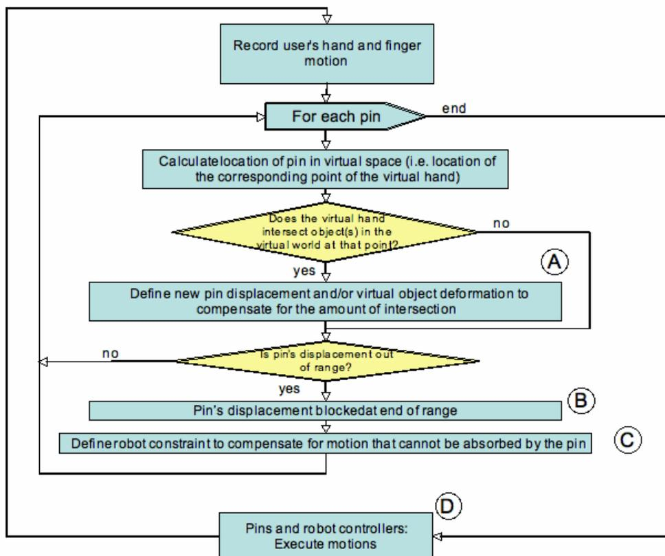
Figure 2. Control program that monitors pin displacement and adjusts the pin and robot controllers to execute appropriate motions to enable the movement of the virtual hand through the virtual space, allowing it to transducer the presence of surfaces and their textures, to edit these surfaces and textures, and to move objects in the space.
