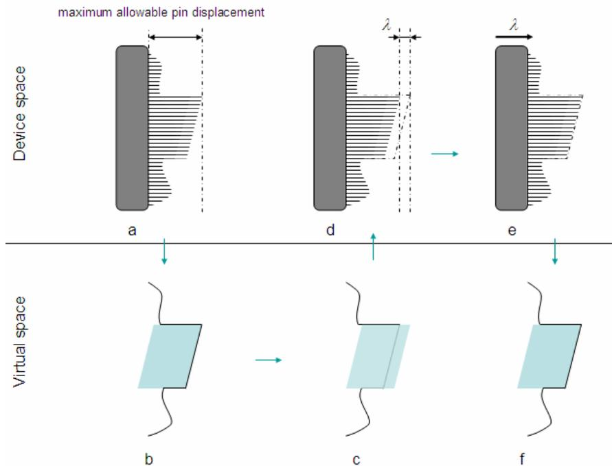
Figure 4. Example of robot motion. When the virtual object creates a displacement greater than can be absorbed by the pin range, the robot arm moves the entire pin assembly. In the case above, the virtual object is moving the hand.
